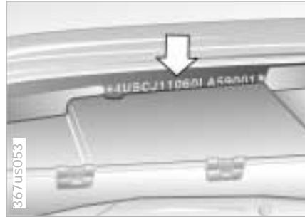
The Vehicle Identification Number is located in the engine compartment below the windshield (arrow) and on the top of the instrument panel.
