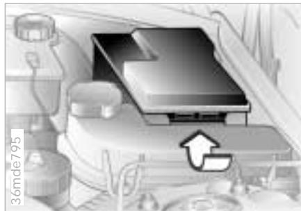
If an electrical accessory fails, switch it off and check the fuse.
