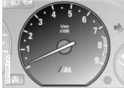
Never allow the engine to operate with the needle in the red overspeed sector of the gauge.
