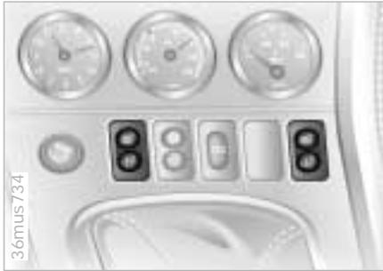
To switch over while heating: press the section of the switch that is dimly lit.
