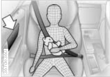
This is the correct way a larger child should sit wearing the safety belt when side airbags (arrow) are provided.
