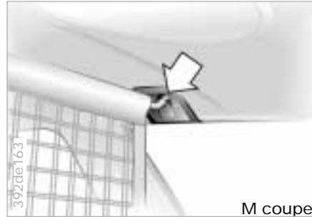
Pull out the partition net on the strap and grip the bar firmly with the other hand. Then grasp the bar on both sides, pull it up and position it into the holders. This process will work out best if you do it from inside the passenger compartment.
