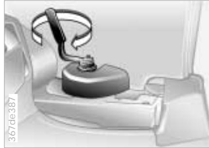
Turn the right and left locking levers of the rear hardtop mounting fasteners in the direction of the arrow to the stop.
