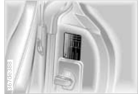
The inflation pressures are indicated on a label attached to the B-pillar behind the driver's door (visible with door open).
