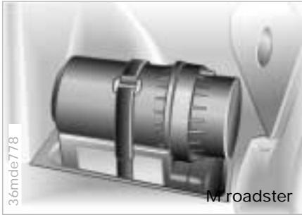
The M Mobility system is located in the luggage compartment at the rear right, on the M coupe also under a cover.
