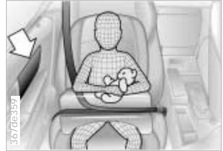
This is the right way a child should sit in a child restraint when side airbags (arrow) are provided.
